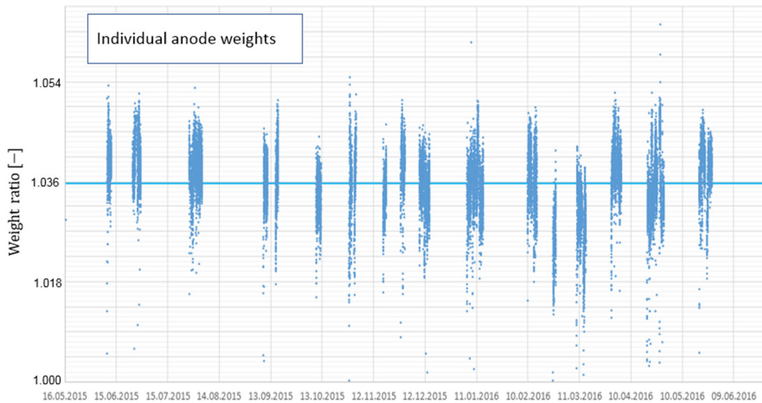
Figure 8. Weight of a specific product produced at compactor C2650 in Årdal from May 2015 to May 2016.
